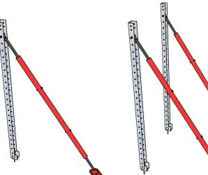
STEP ONE DRILL AND FIX FIRST UPRIGHT TO THE LINE OF THE WALL MINUS THE PLYWOOD THICKNESS. FOLLOW THE MANUFACTURER'S TECHNICAL APPROVAL AND INSTALLATION GUIDES TO PROPERLY SECURE THE CONCRETE
