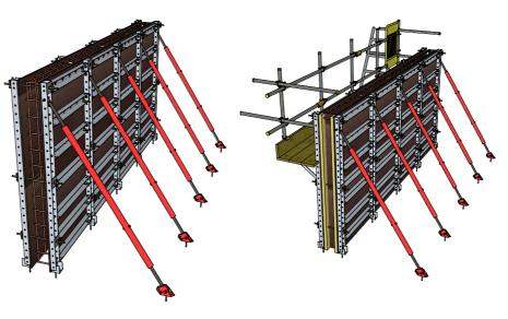
STEP ELEVEN: FIX HANDRAILS / ACCESS IF REQUIRED [REFER TO DRAWINGS FFS-APHR# FOR MORE
