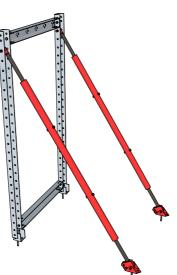
STEP THREE LOOSELY BOLT BOTTOM AND TOP HORIZONTAL JOINING MEMBERS.
