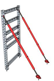
STEP FOUR FILL IN REMAINING HORIZONTAL JOINING MEMBERS.
