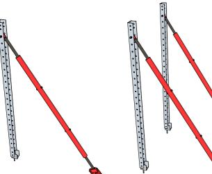
STEP ONE DRILL AND FIX FIRST UPRIGHT TO THE LINE OF THE WALL MINUS THE PLYWOOD THICKNESS. FOLLOW THE MANUFACTURER'S TECHNICAL APPROVAL AND INSTALLATION GUIDES TO PROPERLY SECURE THE CONCRETE
