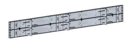
Place a road form pan on top of another road form pan - regardless whether the road form pan is 150mm or 200mm high, the PROCESS REMAINS THE SAME - AND JOIN THEM TOGETHER USING 4X MI2X35MM BOLTS. THE BOLTS MUST BE WELL SECURED AND TIGHTENED USING A SPANNER.
