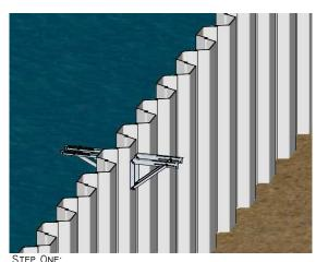
DRILL 2X HOLES IN THE SHEET PILE FOR EACH BRACKET PAIR AT DESIRED HEIGHT (REMEMBER TO TAKE PLY THICKNESS INTO CONSIDERATION WHEN DETERMINING THE LEVEL OF DESIGNED BEAM). OPPOSITE BRACKETS TO BE FIXED WITH BLIND/TENSILE BOLTS WITH ONE OF THE BOLTS POSITIONED AT THE TOP OF THE SLOT OF THE VERTICAL MEMBER. FOR EVERY SEGMENT OF SHEET PILE POSITION TWO PAIR OF BRACKETS AS CLOSE TO THE CORNERS OF SHEET PILING AS POSSIBLE.
