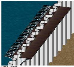
POSITION THE PLY ON THE BRACKETS AND FIX WITH 25MM WOOD SCREWS USING ALL AVAILABLE HOLES. COVER ONE SIDE WITH PLY IN FULL FOR ACCESS AND THE OTHER SIDE JUST ENOUGH TO ACCOMMODATE THE VERTICAL PLY.
